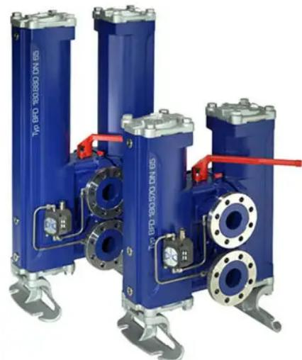
The integrated ball valve switchover makes this filter extremely user-friendly to operate. By simply turning the lever, it is possible to switch back and forth between the two filter housings without having to shut off the medium or change the direction of flow. This function not only saves time during maintenance work, but also ensures that no unwanted contaminants enter the system.
